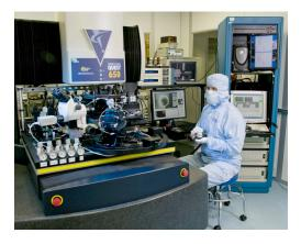
**Robotic assembly machine keeps NIF on target:** LLNL scientists and engineers have developed the precision robotic assembly machine to manufacture the small and complex laser-driven fusion ignition targets for the world's largest and most energetic laser, the National Ignition Facility.
