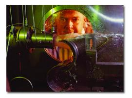
Hot stuff: A Laboratory technician peers at an experimental apparatus used to analyze nozzle and turbine-blade designs. A geothermal turbine was developed at Livermore for generating energy using the flow of liquid and vapor from geothermal wells. Researchers tailored nozzles and turbine blades for maximum efficiency and operation in hot, corrosive brines.
