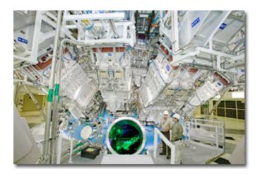
Bird's eye view: A view into the National Ignition Facility target chamber of the Final Optics Damage Inspection (FODI) system -- used to monitor the condition of the final optics in the NIF beamlines.
