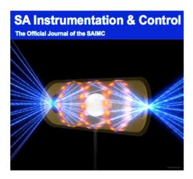
This artist's rendering shows a National Ignition Facility target pellet inside a hohlraum capsule with laser beams entering through openings on either end.
