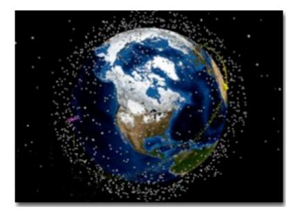
A visualization generated by Ming Jiang, of LLNL's Computation, shows the simulated debris from an exploded satellite in the lower Earth orbit, along with active satellites positioned using a semi-analytical orbital propagator.
