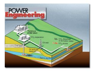
One approach to help stem the increase of carbon dioxide in Earth's atmosphere is to capture it at the source and inject it into an underground formation.
