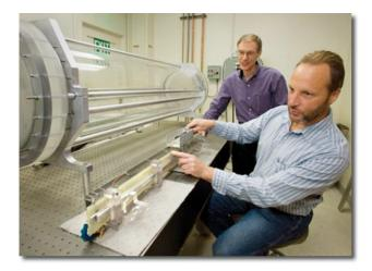
Engineer Mark Rhodes (seated) and physicist George Caporaso adjust a prototype Blumlein transmission-line generator, which will supply power to the high-gradient insulators forming the beam tube dielectric walls in LLNL's compact proton accelerator.
