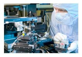
**Right on target:** The National Ignition Facility's millimeter-sized targets must be designed and fabricated to meet precise specifications for density, concentricity and surface smoothness for NIF experiments. LLNL scientists and engineers like Richard Montesanti have developed the precision robotic assembly machine to manufacture the small and complex laser-driven fusion ignition targets.
