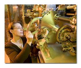
**Load 'em up:** Susan Zimmerman, a postdoctoral student, loads a sample of sediment in the Lab's large accelerator for mass spectrometry (AMS). The AMS uses isotopic ratios of carbon-14 to date the samples. Zimmerman and colleagues are studying records of drought over the last several thousand years preserved in California lakes.
