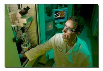
Picture perfect: Selim Elhadj mounts a sample and makes adjustments to image individual spores with an atomic force microscope (AFM).
