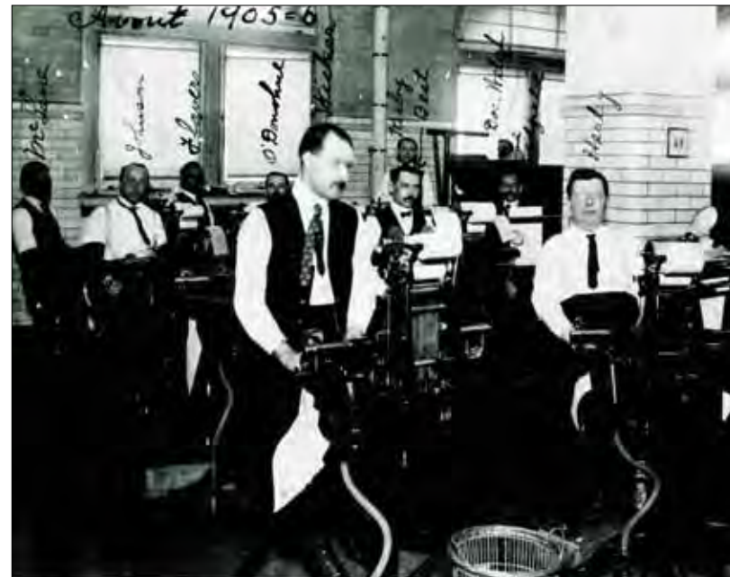
The first battery of Monotype keyboards, 1905: The “weird machines that set type by punching holes in paper.” This modest group rapidly grew.
