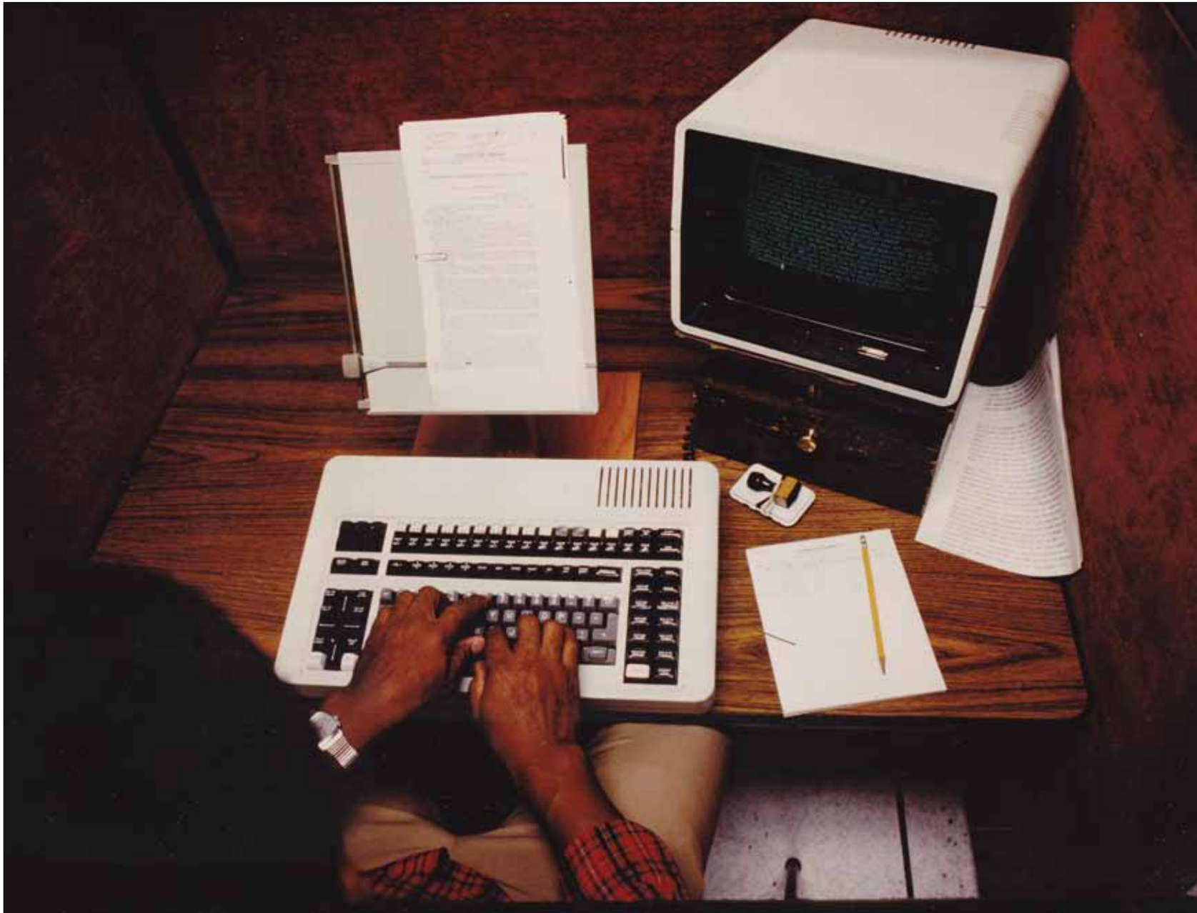
Terminal for the Atex photocomposition system, Electronic Photocomposition Division.
