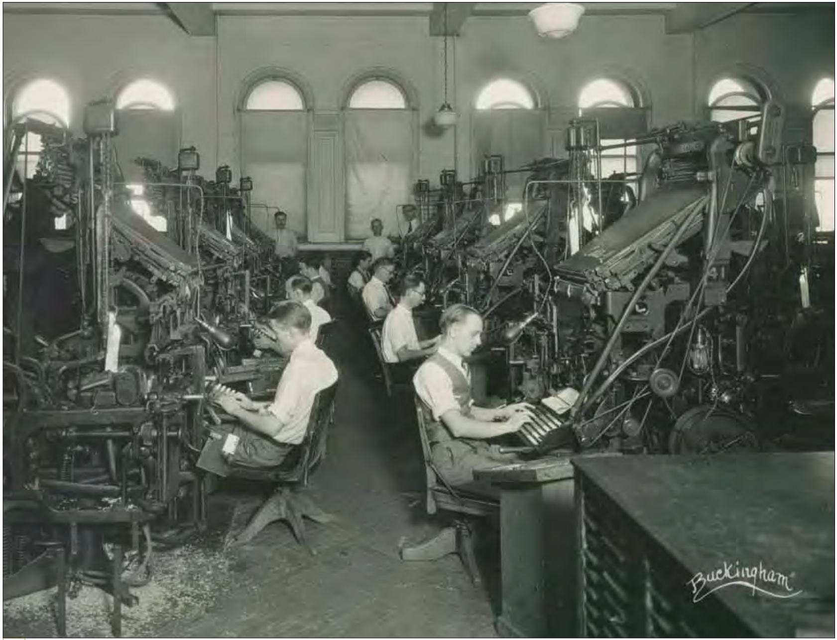
An early shot of the Linotype battery, probably ten years after their introduction in 1904.
