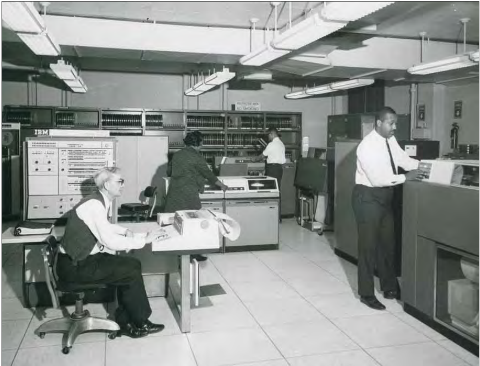
GPO launched itself into the computer age with the Linotron, a magnetic tape typesetting system developed under a GPO contract by the Mergenthaler Co. and CBS Laboratories.
