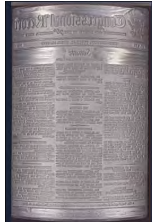
The last issue of the Congressional Record printed from stereotype plates struck from lead type, April 10, 1979. Hot metal typesetting ended altogether in 1985.
