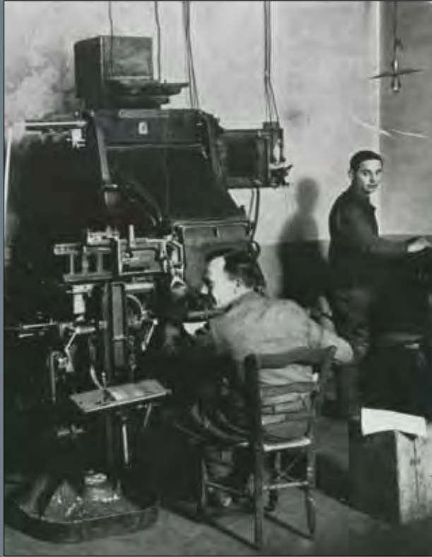
The Model 5 Linotype machine in Chaumont, France, with Corporal Jimmie Kreiter of the 29th Engineers Battalion at the keyboard.
