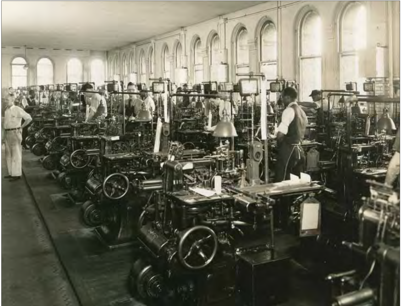
Monotype casting machines, part of the revolution that changed the typesetting formula from minutes per line to lines per minute.
