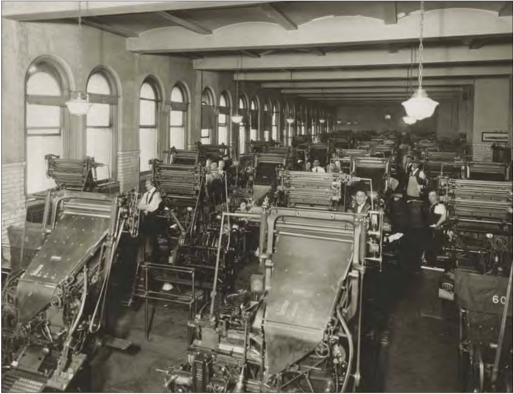
GPO had one of the biggest batteries of Linotype machines in the world.
