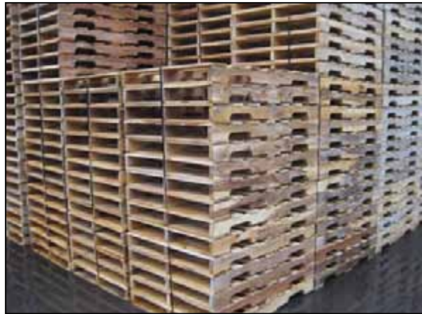
Figure 3.21. ~ Stringer pallet design.
