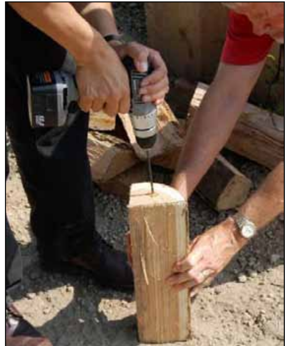
Figure 4.13. ~ Drill a hole in the firewood to accommodate a temperature sensor. Drill a hole from the side at midsection for a thermocouple (left). Drill a hole from the end for a probe (right).
