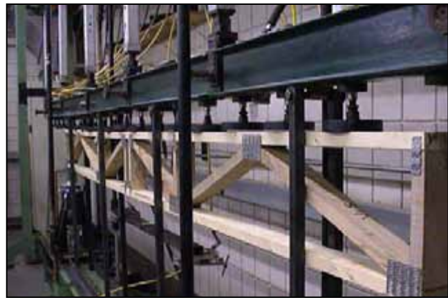
Figure 3.32. ~ Floor truss on a testing rack.
