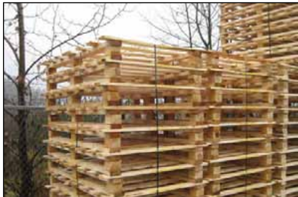
Figure 3.22. ~ Block pallet design.
