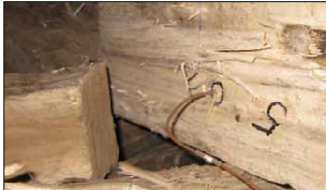
Figure 4.15. ~ A thermocouple wire secured in the firewood.
