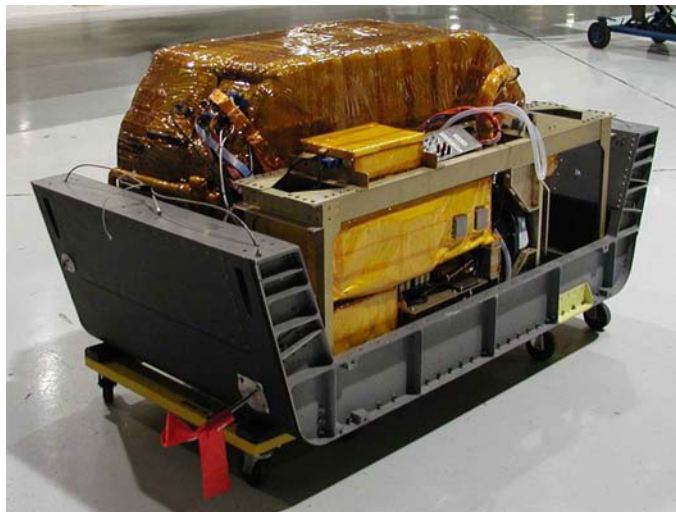
Figure 1. The Harvard ICOS instrument integrated into the WB-57 pallet is shown on the left. The schematic on the right shows the principal of operation of the ICOS technique.
