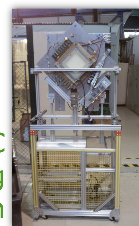
4 MWPC Tracking System
