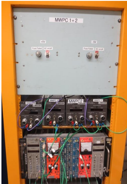
+5V and -5V power supply for N-277 cards
