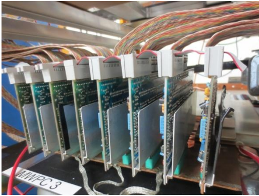
N-277 cards connected to wire plane
