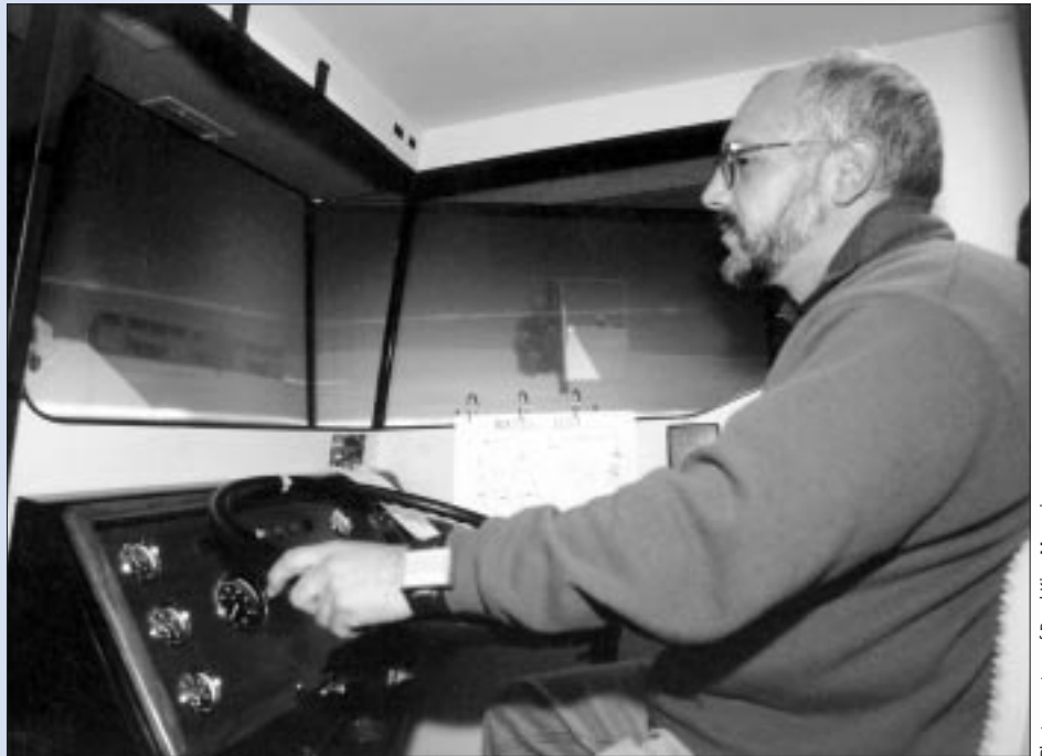
The study used a driving simulator to examine driver performance in challenging, crash-likely driving conditions. On the road, crash-likely situations are rare, but can be induced more frequently, without risk, in a simulator.
