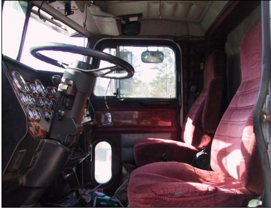
Figure 10. Interior Photo of the Principal Other Vehicle (Crash Partner) Showing no Steering Deformation Source: LTCCS 2000–2003 data.
