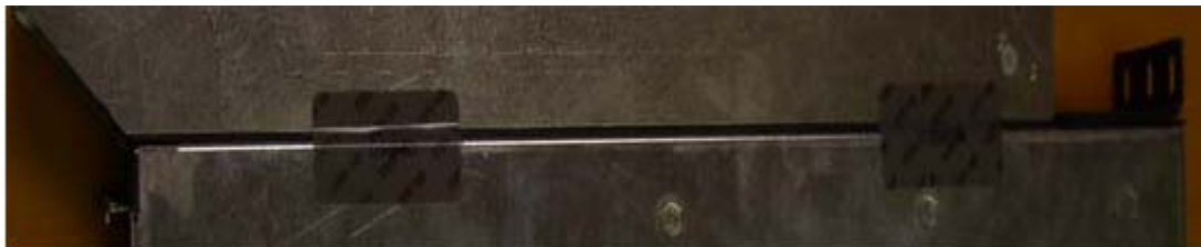
Figure 4 Placement of Opacity Baffle (Bottom View)
