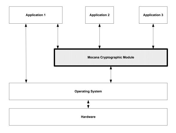
Figure 1 – Cryptographic Module Interface Diagram
