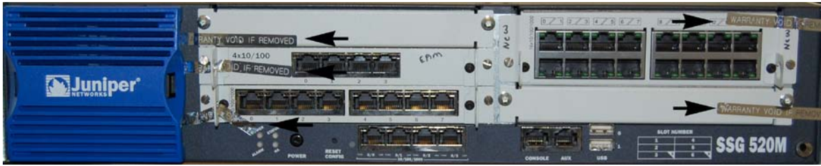
Figure 2: Front of the SSG 520M device, with location of tamper evident seals
