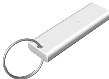
Figure 2: PIV Token Includes a smaller antenna for contactless communications and replaces the golden contact plate with a USB plug to remove the need of a smart card reader.
