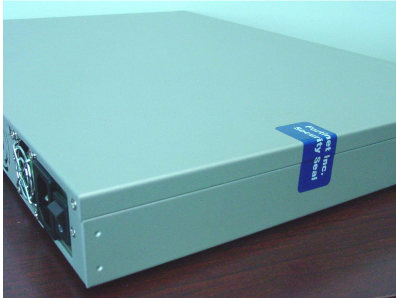
Figure 7: FortiGate-800 tamper seal placement
