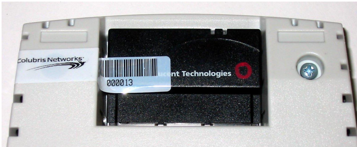
Figure 5 - Placement of Tamper-Evident Seal on Wireless LAN Card and Enclosure
