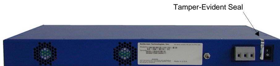
Figure 2 Tamper-Evident Seal on DC Interface
