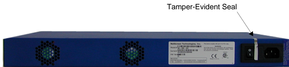
Figure 1 Tamper-Evident Seal on AC Interface
