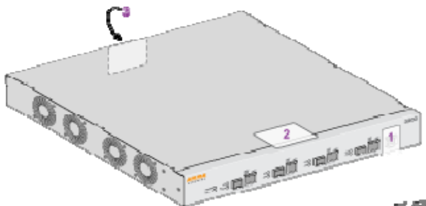
Figure 5 Required TELs for the Aruba 3000-series Controller
