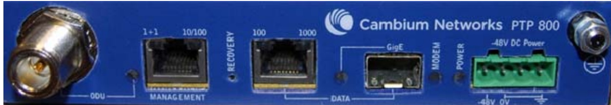
Figure 2 – PTP 800 CMU Front Panel
