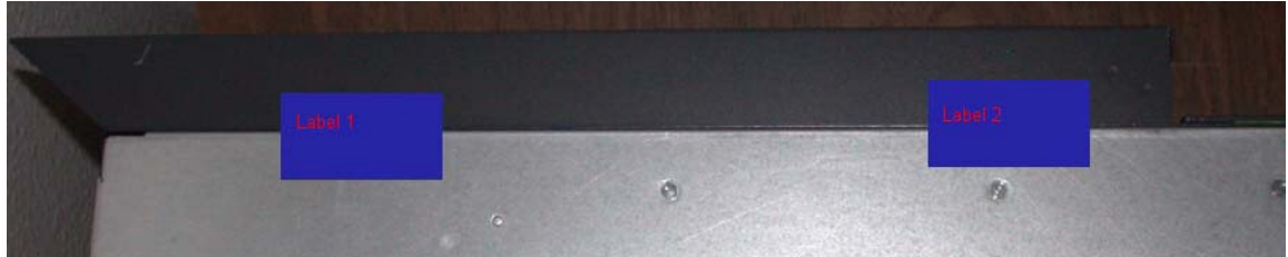
Figure 4 Placement of Opacity Baffle (Bottom View)
