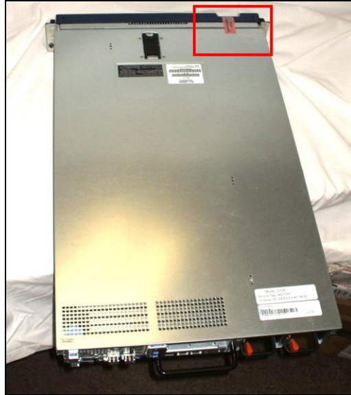
Figure 6 – Tamper-Evident Seal Application Position (Front Bezel)
