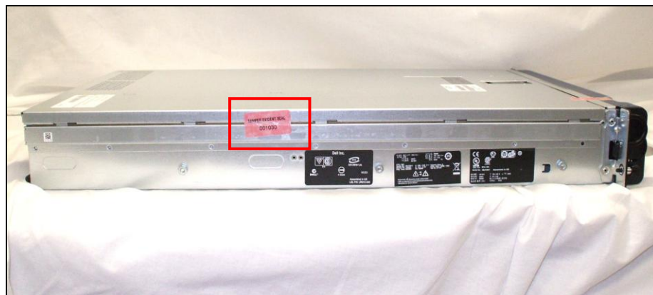
Figure 7 – Tamper-Evident Seal Application Position (Top Cover)
