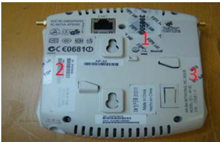
Figure 9 - Aruba AP-92 Tel placement bottom view
