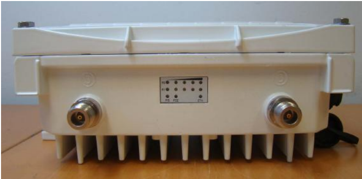
Figure 26 - Aruba AP-175 Tel placement back view
