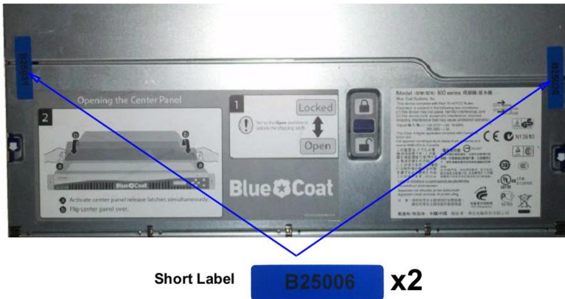
Figure 10 Tamper Evident Label Application – Top of Appliance
