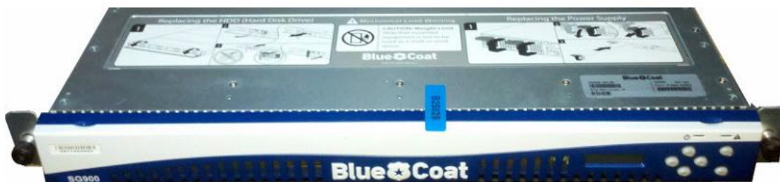
Figure 11 Tamper Evident Label Application – Front Bezel
