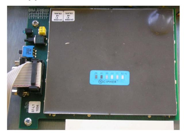
The following figure shows the module mounted inside the NetHSM
