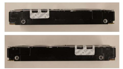
• Security labels on side of drive to provide tamper-evidence of HDA cover removal,
