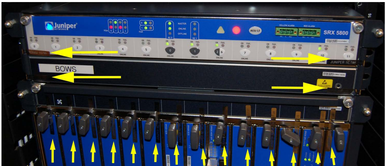
Figure 4. SRX5800 Tamper Evident Seal Location (Front)
