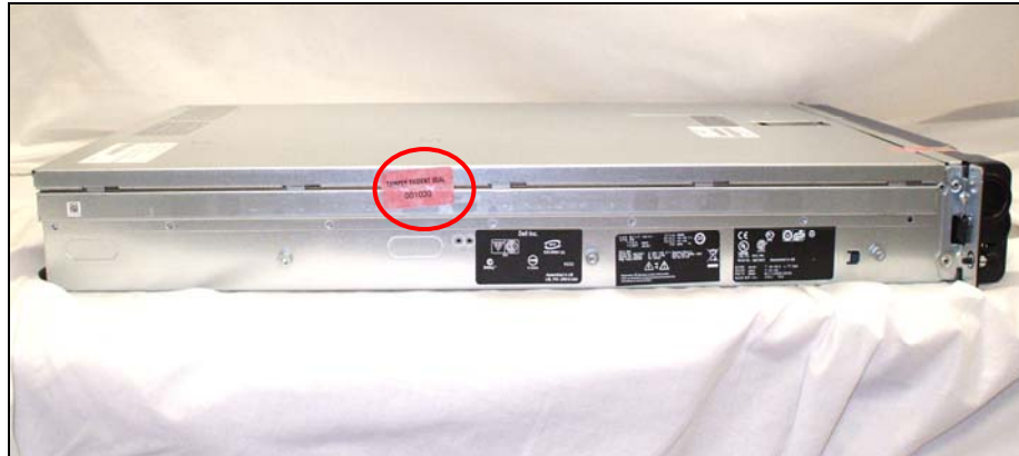
Figure 4 – Tamper-Evident Label Application Instruction at the Right Side
