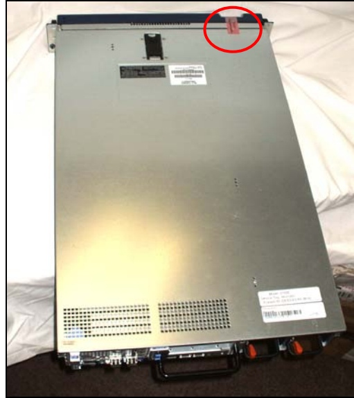
Figure 3 – Tamper-Evident Label Application Instruction at the Front
