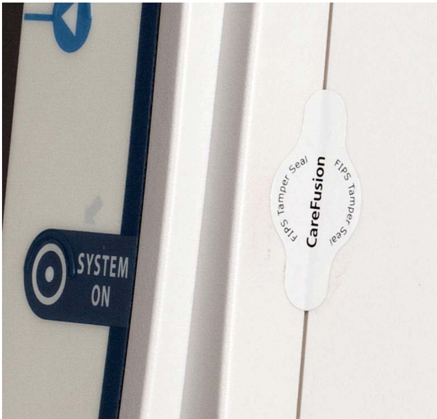
Figure 18 Ensure seal is centered between grooves
