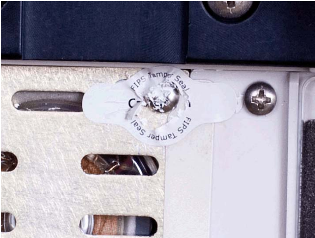
Figure 28 Seal has been gouged out
