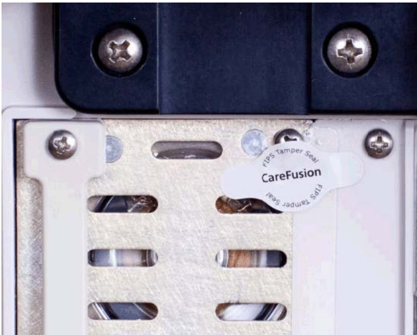
Figure 5 Incorrect seal application
