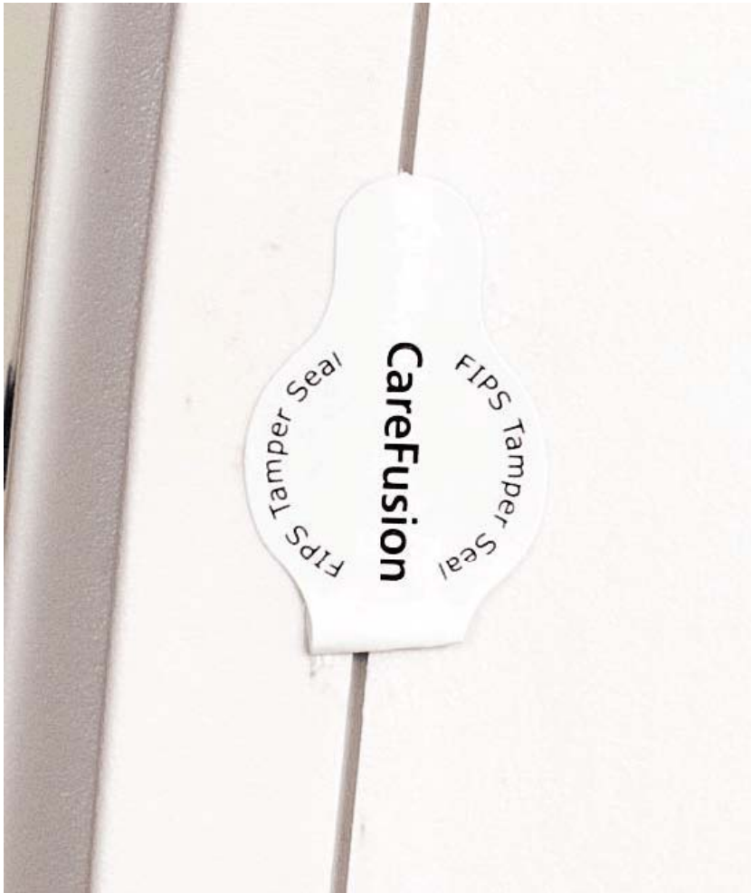
Figure 30 Seal has not been applied correctly; not FIPS compliant
