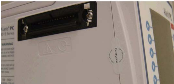
Figure 2 Location of seals on device
