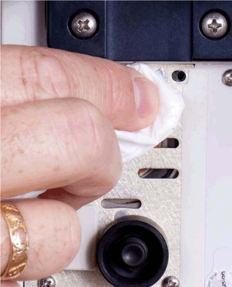
Figure 23 Removing remaining debris
