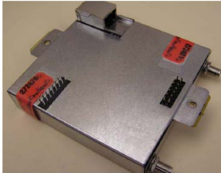
Figure 3 – 3e-523-F2 with tamper seals
