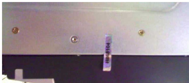
Figure 6 – Tamper-Evident Label Placement (Front Bezel/Chassis)
