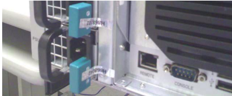
Figure 7 – Tamper-Evident Label Placement (Power Supplies)
