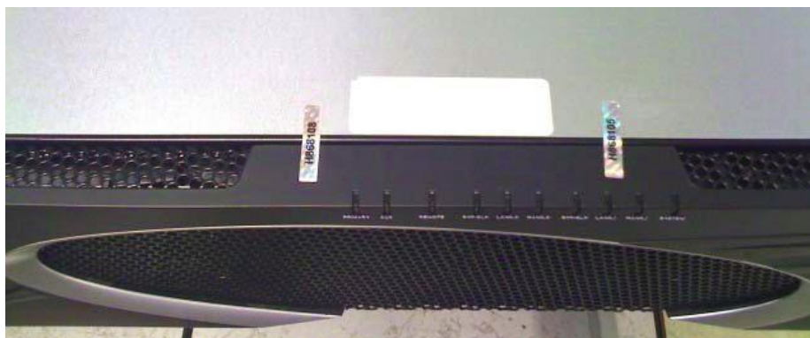
Figure 5 – Tamper-Evident Label Placement (Front Bezel)
