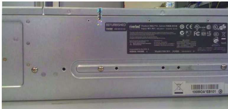
Figure 8 – Tamper-Evident Label Placement (Chassis Cover - right)
