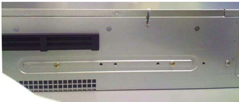
Figure 9 – Tamper-Evident Label Placement (Chassis Cover - left)
