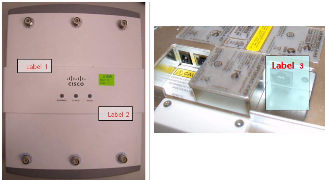
Figure 4 Tamper labels on AP1252
