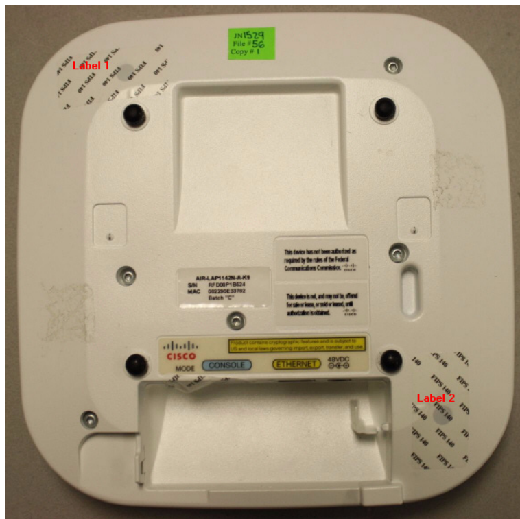
Figure 6 Seals covering screws on module enclosure
