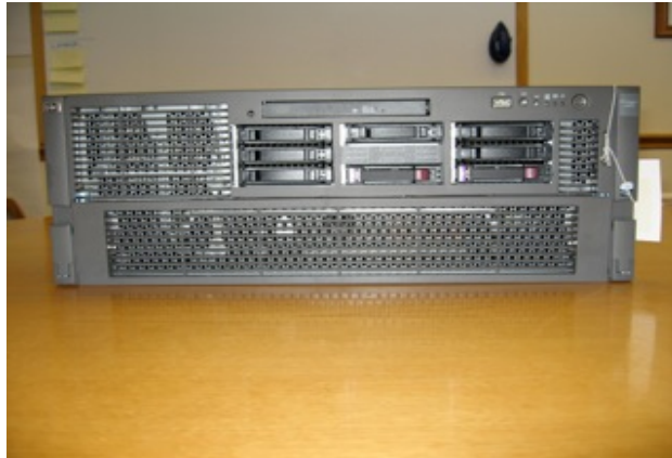
Illustration 7: front plastic cover is vented. Aluminum cage behind plastic has small vent holes.
