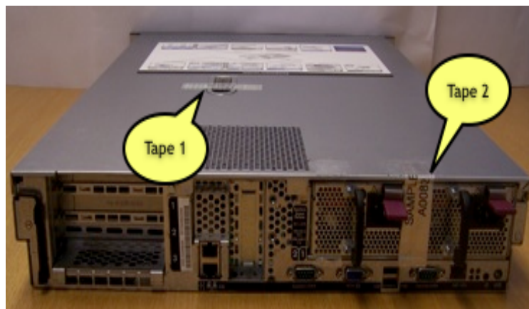
Illustration 4: tamper-evident security tape covering lock and cover latch, two power supplies
