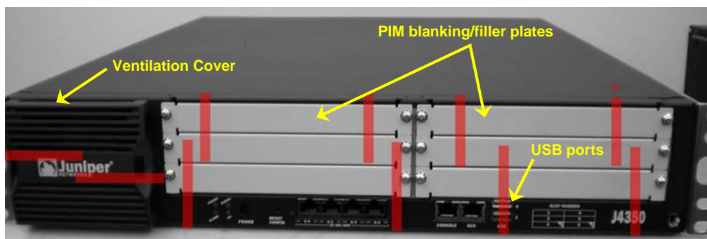
Figure 5. J4350 and J6350 Tamper Evident Seal Location for the Front (10 total)
