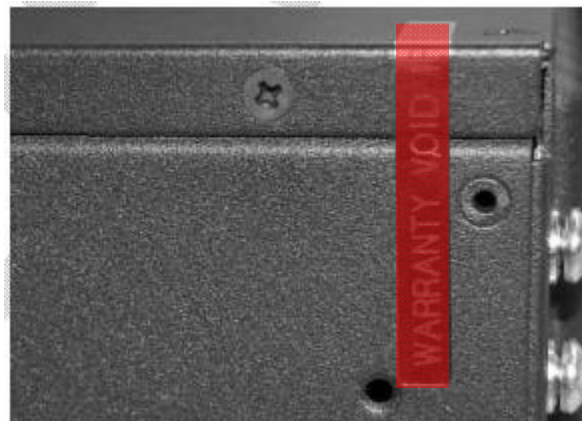
Figure 8. J4350 and J6350 Tamper Evident Seal Location for Rear Corner- Opposite Power Supply (1 total)
