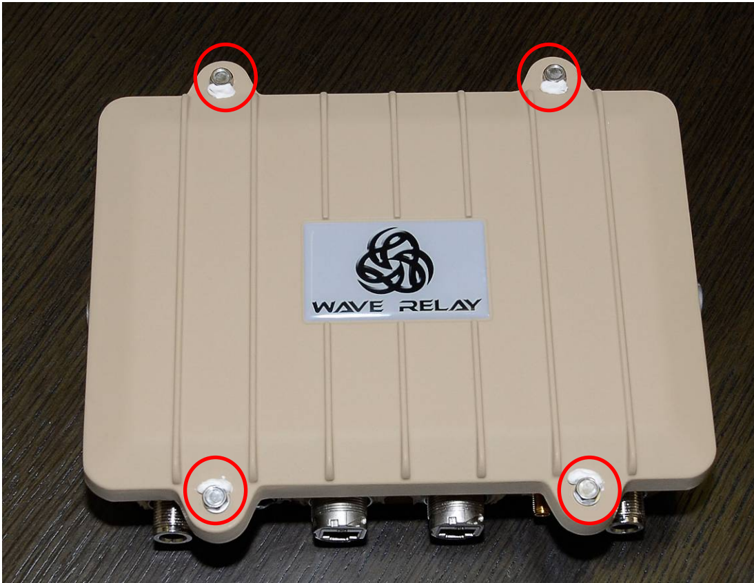
Figure 6 – Tamper-evident material placement for Quad Radio Router Cover (4 locations indicated by red circles)
