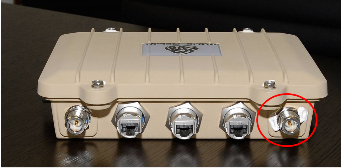
Figure 7 – Tamper-evident material placement for Quad Radio Router Wireless Radio Port (Top – 2 locations indicated by the red circle)
