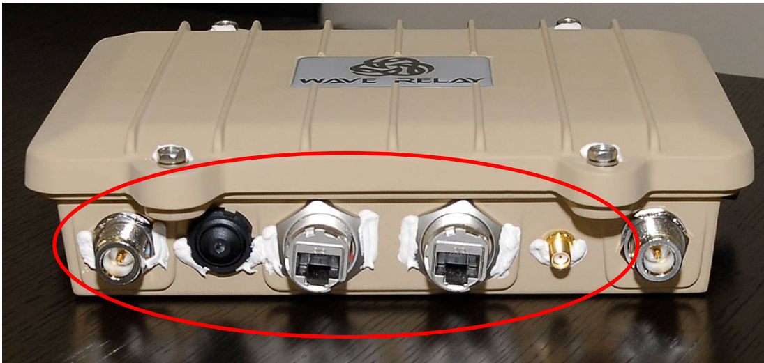
Figure 8 – Tamper-evident material placement for Quad Radio Router Bottom (9 locations indicated by the red circle)
