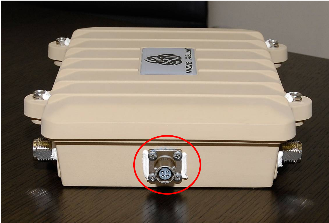
Figure 9 – Tamper-evident material placement for Quad Radio Router Serial Port (Left – 2 locations indicated by the red circle)
