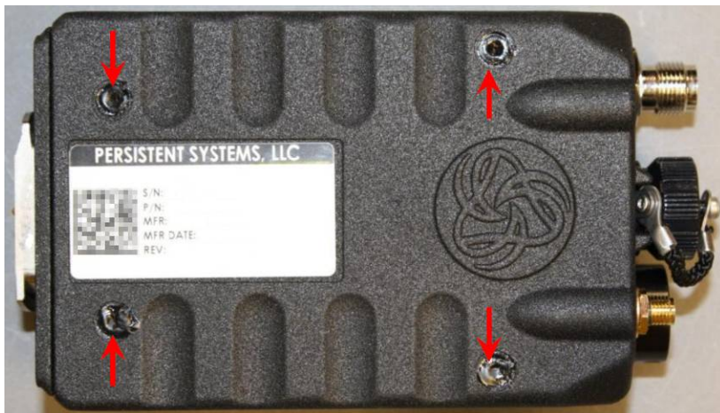
Figure 5 - Tamper-evident material placement for MPU4 (4 locations indicated by red arrows)
