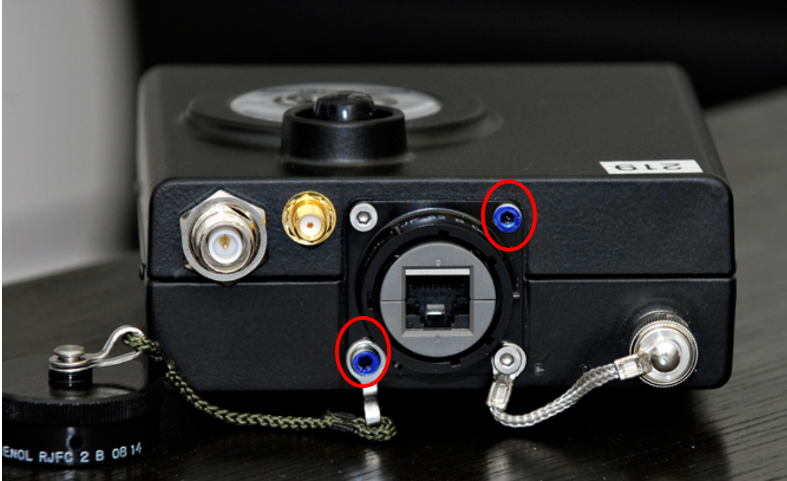
Figure 2 – Tamper-evident material placement for MPU Top (2 locations indicated by red circles)
