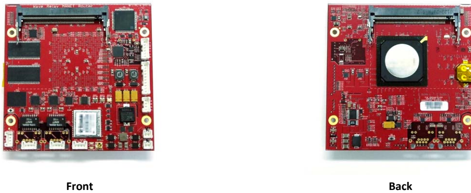
Figure 2 – Physical Boundary of Wave Relay Dual Radio Board
