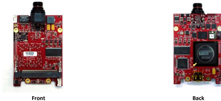
Figure 1 – Physical Boundary of Wave Relay Single Radio Board
