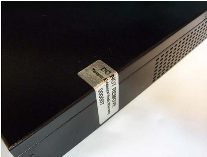
Figure 5. Tamper evident seal is located on the left side panel
