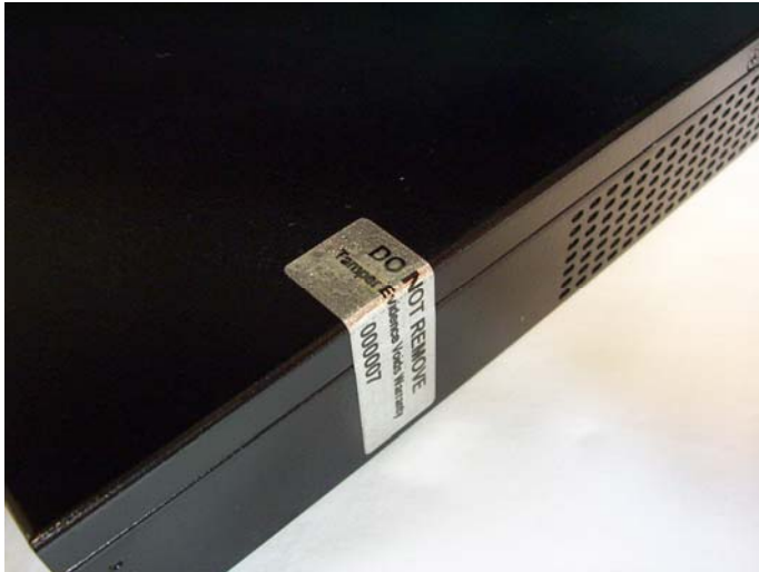
Figure 6. Tamper evident seal, located on the left side panel
