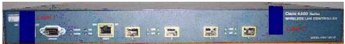
Figure 1 Placement of Tamper-evident Labels (Front View)
