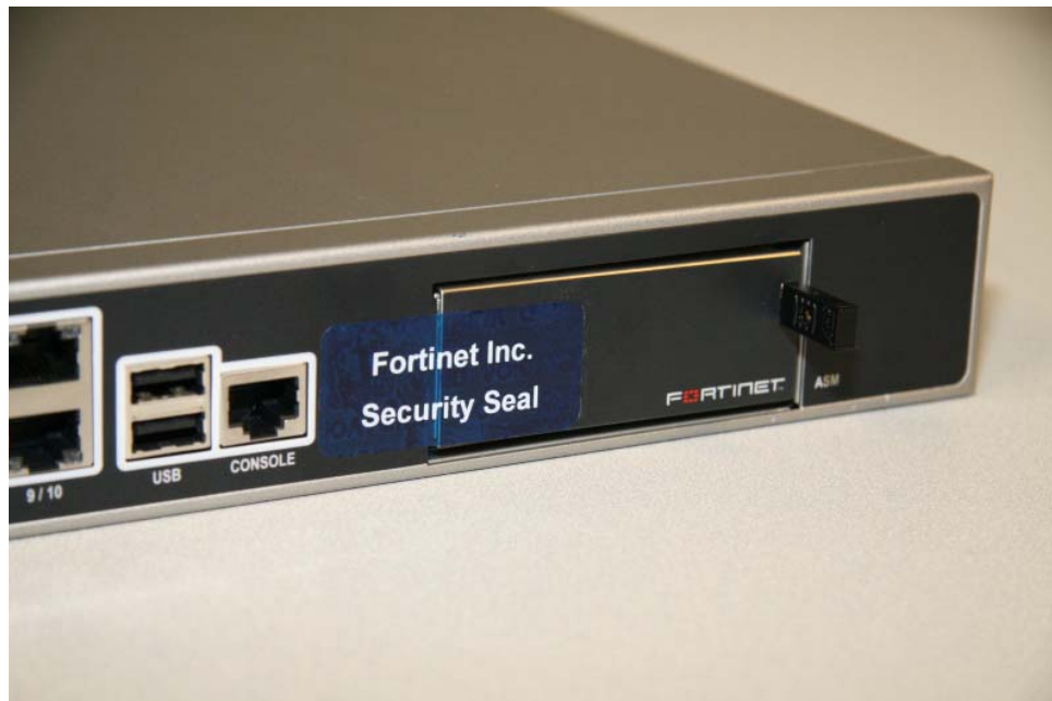
Figure 4: FortiGate-310B AMC faceplate seal
