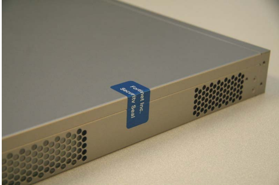
Figure 3: FortiGate-310B external enclosure seal
