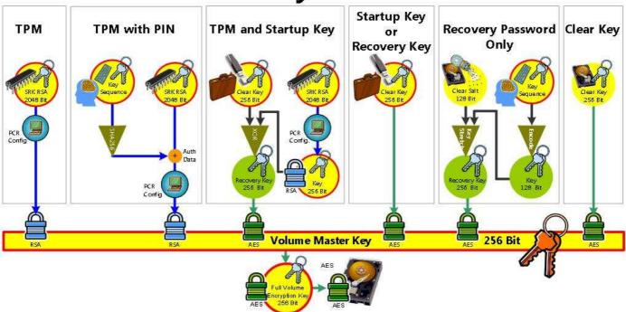
In Server 2008, triple-factor authentication has also been added. The diagram below shows the architecture of the new authenticator.
