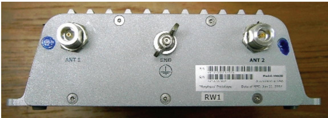
Figure 6: Rear View of the SWAB Hardware (ES520V2) Showing the Blue Thread Locker
