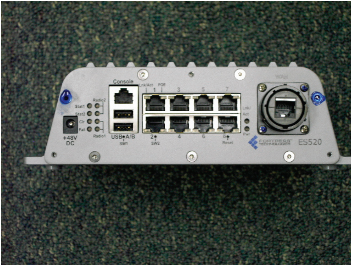
Figure 3: Front View of the SWAB Hardware (ES520V1) Showing the Blue Thread Locker
