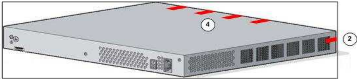
Figure 13 – Cisco 2801 Tamper Evident Label Placement (Back View)
