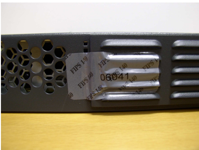
Figure 9 Tamper evident label attached on the opacity shield of Router 2801
