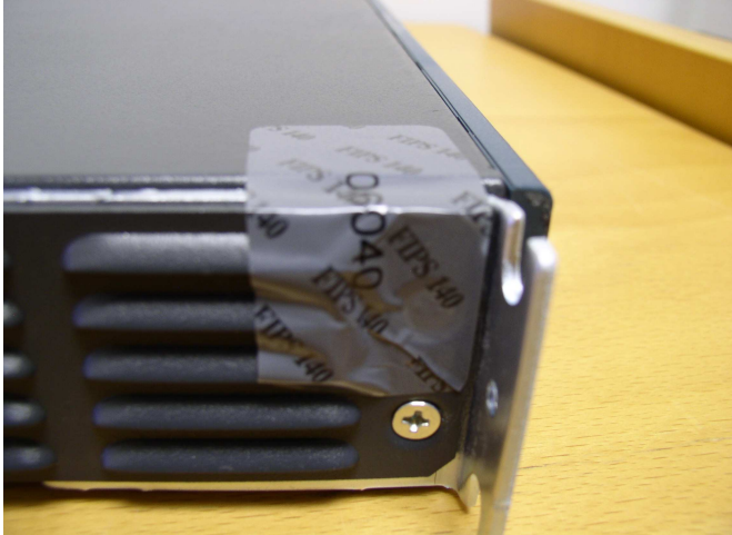
Figure 10 Tamper evident label attached on the opacity shield of Router 2801
