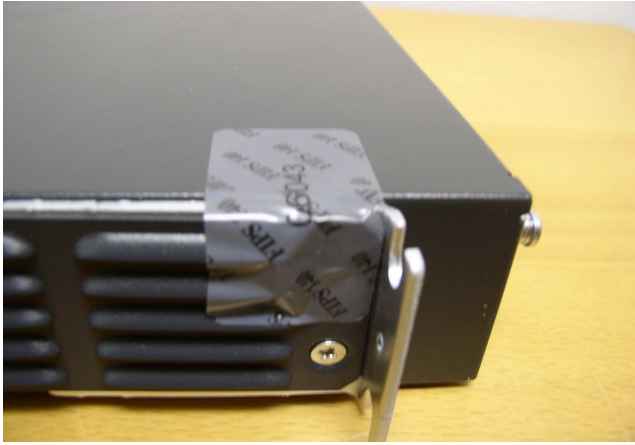
Figure 7 Tamper evident labels attached on the opacity shield of Router 1841
