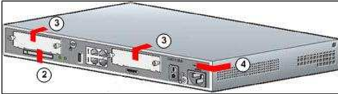
Figure 11 – Cisco 1841 Tamper Evident Label Placement (Back View)
