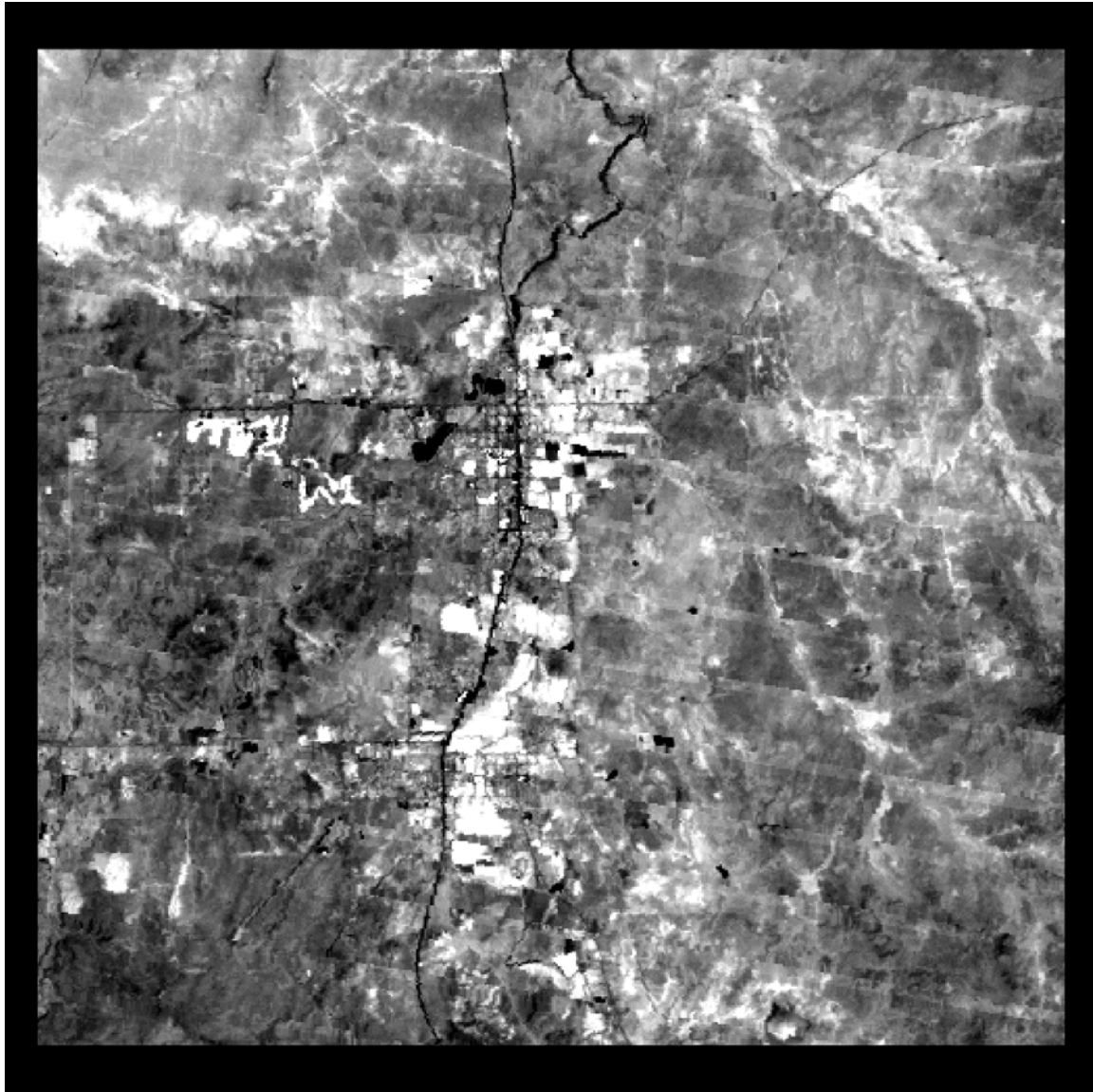
Figure 31. ETM+ Band 4 subset of scene shown in Figure 1 after filling in the blanks with digital numbers derived from regression tree analysis.
