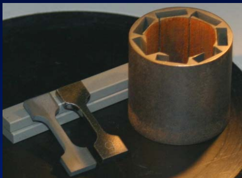
25 mm long with gauge section of 2 x 2 (mm 2 )
